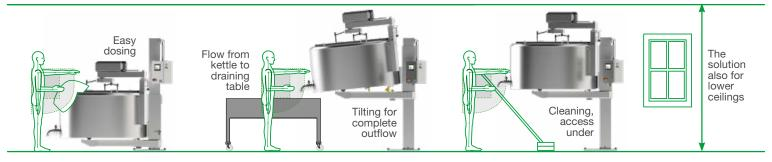
Note: the elevating device, displayed in the graphics above works with the principle of hydraulic aggregate. The advantages are the same for the new elevating device.
