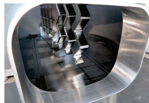
Rake stirrer with slotted filter bottom in LC
