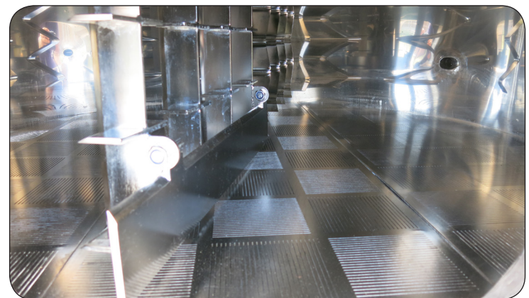
Rake stirrer in lauter cistern, line cut filter bottom
